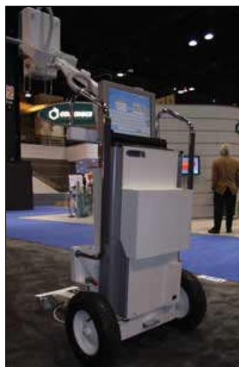
iCRco Inc. debuted its Vertex system at RSNA 2008, spotlighting its "True Flat Scan Path" software, intended to eliminate the use of rollers to transport the phosphor plate across the scan head, resulting in an artifact-free image. (iCRco)
